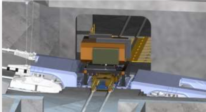
Upper station with HLW transfer cask
