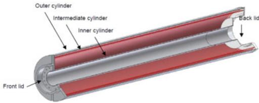
Figure 4. Heater element general design (Aitemin).
