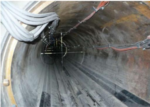
Figure 8. View of the convergence instrumentation in the insert.
