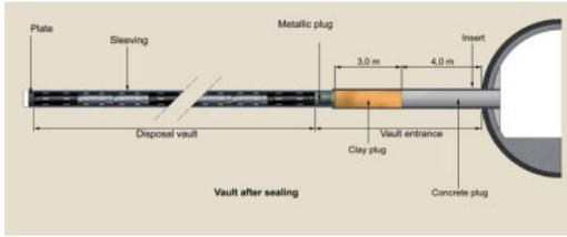
Figure 1. Concept of disposal cell for HL-LL activity waste.
