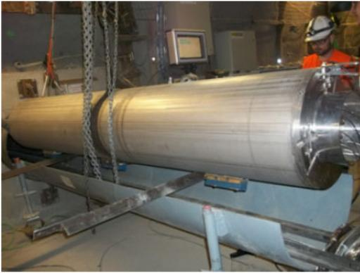
Figure 7. Positioning of a heater element at the cell entry before insertion.
