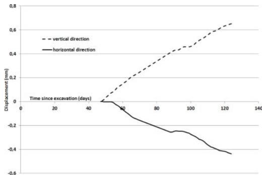
Figure 11. Sleeve diameter evolution at 8 m depth – positive displacement corresponds to extension, negative to compression.
