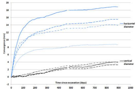
Figure 3. Convergence measured along horizontal and vertical direction in an unsleeved 20 m long cell (Phase 1b) – full line: 16 m depth; dash line: 12 m; dash/dots: 8 m; dots: 4 m.
