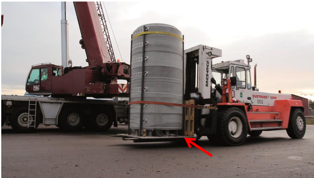
Figure 3. A fully assembled distance block, the cable block can be seen at the bottom of the component (marked with a red arrow).
