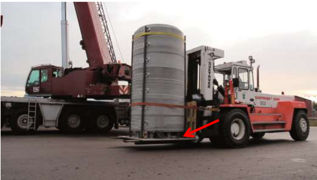
Figure 1.9 Test distance block being moved out from the assembly facility. The red arrow marks part of the sensor arrangement, a cable block, in which sensor cabling can be placed during transport and deposition.
