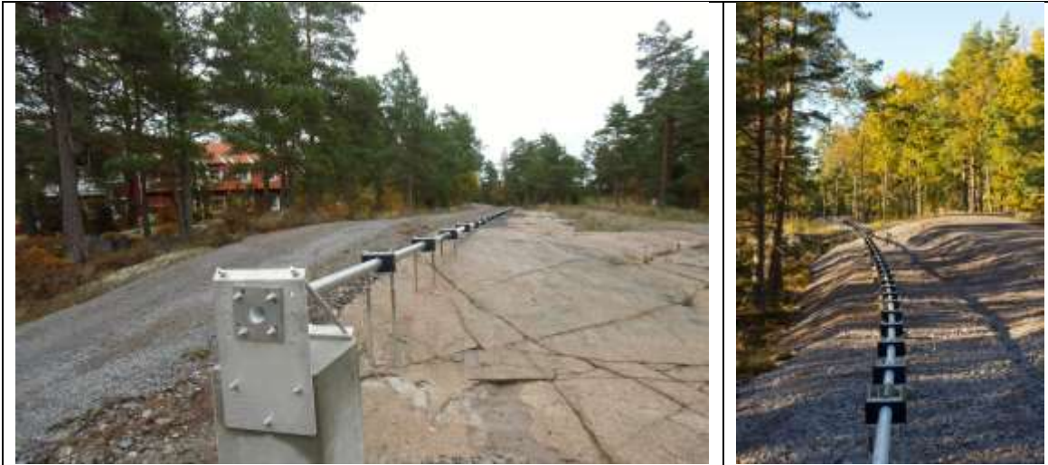
Figure 1.12. Äspö deviation control facility is a 300 m long plastic tube ( \varnothing 75 mm) secured firmly to the ground with 151 fastening devices. All material used in the construction is non-magnetic such as plastic and aluminium.
