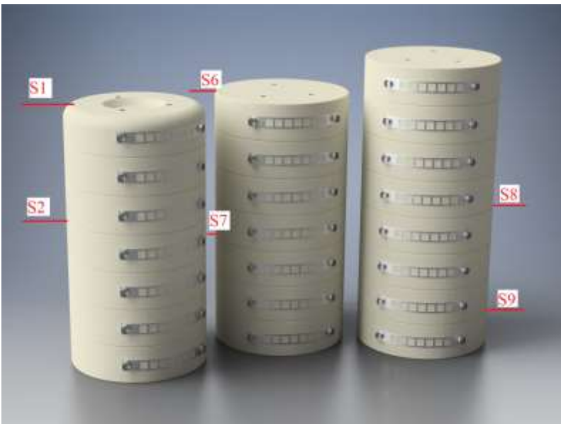
Figure 1.8 Schematic illustrations of the distance- and transition blocks with their feet. Positions used for instrumentation in the MPT are marked, S1-S9.
