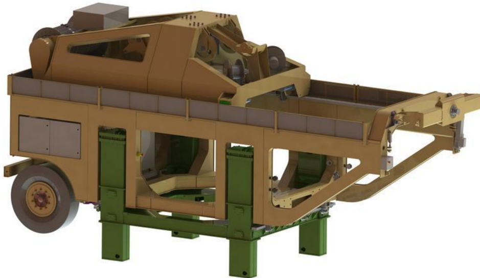
Picture 1. Buffer block installation machine
