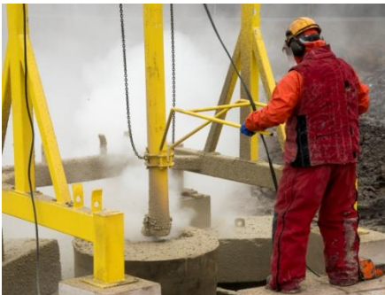
Fig. 7 Testing of water jet excavation on the surface.
