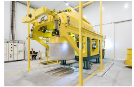
Fig. 2 Buffer installation machine (BIM).
