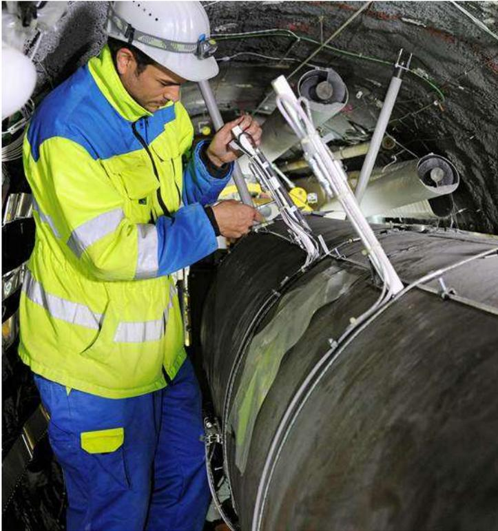
Heavily instrumented heater (with erectable sensor holders) and the backfilling machine in the background © COMET
