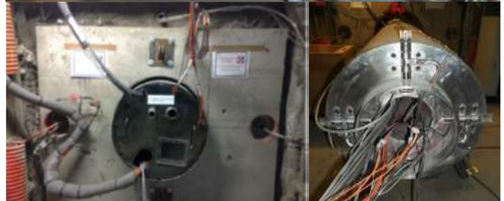
Installation of the heaters in the ALC-experiment in Bure
